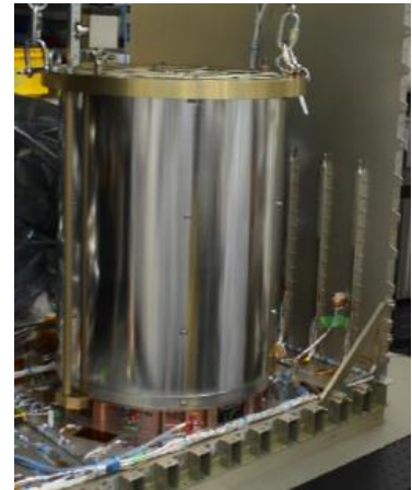
Fig. 1: SHM installed (with holding tool) into the ACES payload at Airbus.
